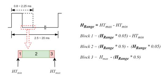
The PWM input controls motor startup and speed regulation:
