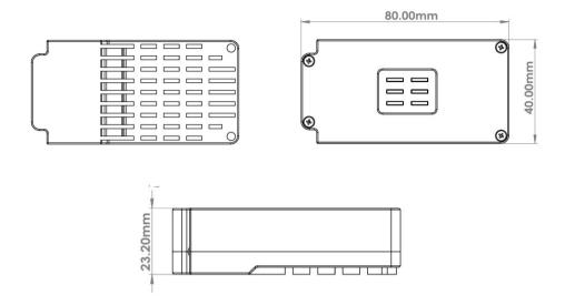
The external dimensions of the **ACD-V04B120A** are illustrated in the following drawings. Typical dimensions are provided below for reference purposes.
