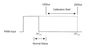
The diagram illustrates the method for entering **calibration mode**. After power-on, the controller enters the **Automatic Detection** state, where it monitors the input signal. If the detected throttle signal remains within the "**Calibration Start**" region in the diagram for at least **2 seconds**, the system will enter calibration mode.
